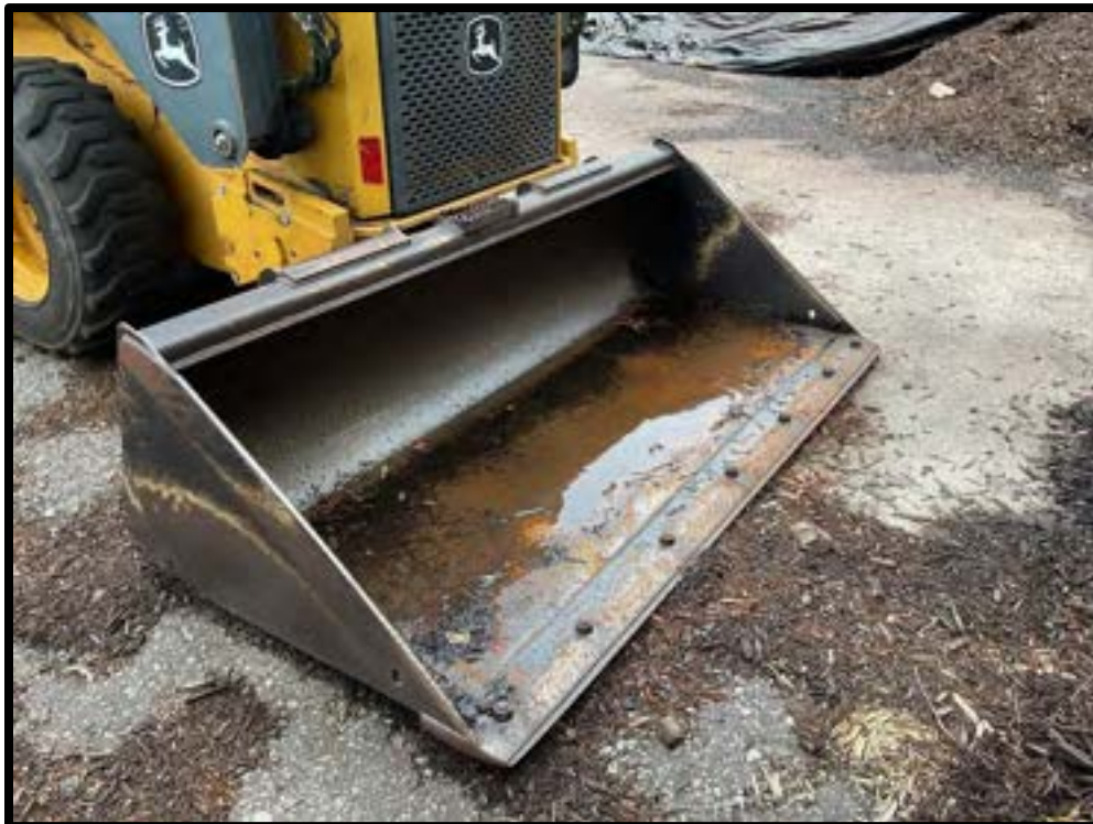
Photo #5: Water accumulated in equipment
